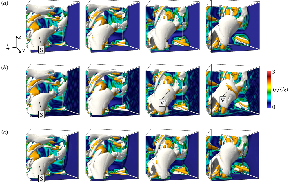
Figure 6: Temporal evolutions of small-scale shear layers and vortex tubes at different time instances ( \tau/\tau_{\eta P} = 1.3, 3.7, 5.5 and 7.3 ) progressing from left to right in each panel: (a) R350, (b) R350L30e and (c) R350L210e. The shear layers (grey) and vortex tubes (orange) are visualised respectively by the isosurfaces of shear intensity I_S = 1.5\langle I_S \rangle and rigid-body-rotation intensity I_R = 3\langle I_R \rangle , with averages used as reference values taken at the flow centre. The visualised domain is a cube of size L_0^3 , with the walls coloured by I_S .
